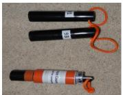
Dibbers - **Special 68** has a fat marker/identity tube fitted (top one in picture – may be all white). This can be used to check that a Triffid is working or how many dibs have occurred. Before the event this should be zero. It will not create a log entry, has no effect on event data.
